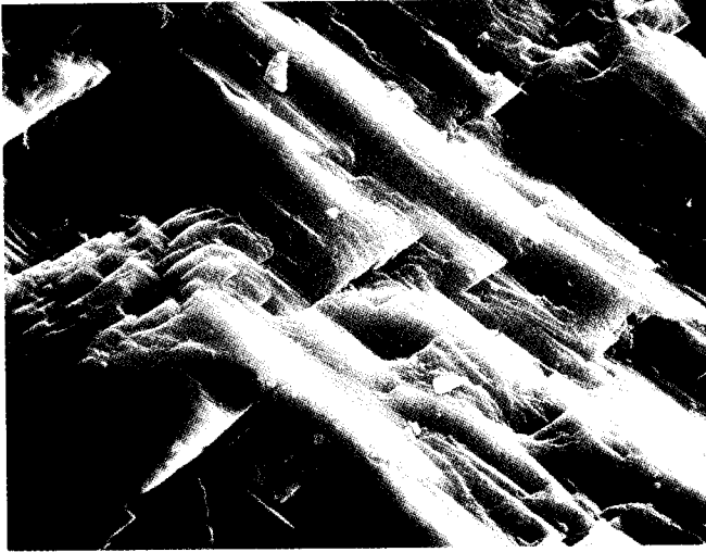
Figure 2—Scanning electron photomicrographs of reacted K-feldspar grain surfaces in several different solutions: (A) from experiment 1 in sodium chloride, (B) from experiment 2 in sodium acetate, and (C) from experiment 6 in acetic acid. Magnification = 2000 \times .
